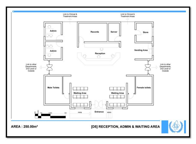
FIG. 1. Typical layout of the main reception area.
